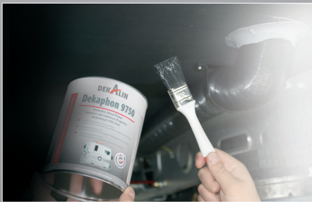
Protection of wooden plywood (floor) panels
