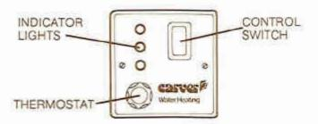
BEFORE SWITCHING ON make sure that water flows from the hot taps. This indicates that the water heater is full. Check that the gas and electrical supplies have been connected and turned on.
