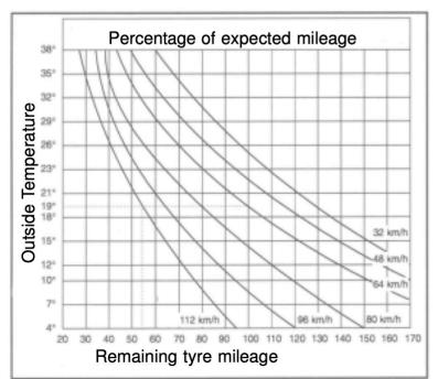
Excessive speed and high temperature also contribute to increased tyre wear.
