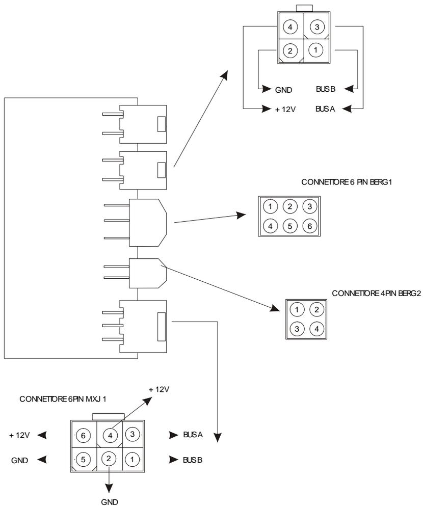
Figure 12 "Layout of Node Connectors"
