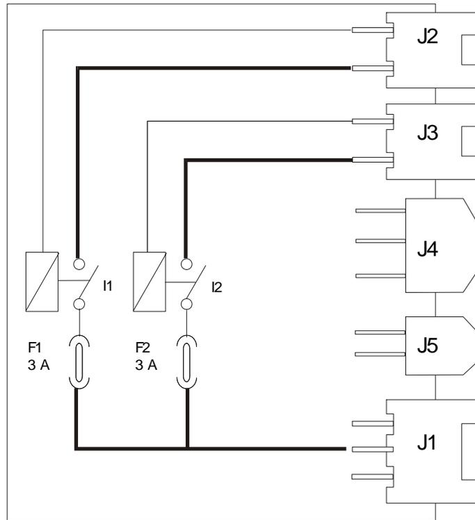
Figure 13"Node equivalent logic layout"
