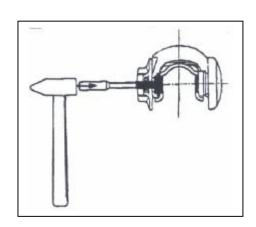
If this does not rectify the problem long term, telephone AL-KO and request REPLACEMENT RATCHET WHEEL. This modified wheel has the centre spindle threaded only half way and allows the ratchet wheel to spin freely once released.
