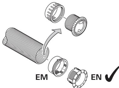
**i** The new end outlet and the old end outlet nut (and vice-versa) cannot be combined.
