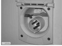
Fig. 110 230 V connection on vehicle
