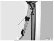
Fig. 53 Hinged window with rotary hinges, open
