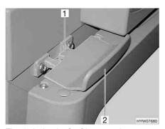
Fig. 159 Lock of refrigerator door, closed (Thetford)
