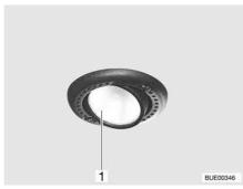
Fig. 215 Recessed halogen light
