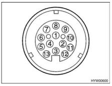
Fig. 115 Contact diagram of the thirteen-pin plug
