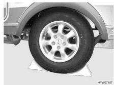
Fig. 232 Securing support wheel
