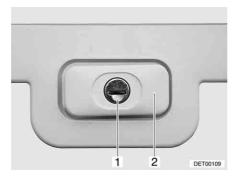
Fig. 30 Flap lock, rectangular, closed
