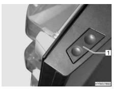
Fig. 155 Release button of the refrigerator door (Dometic 8 series)
