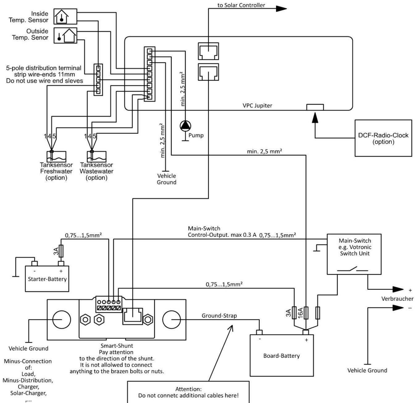
All terminals are designed in such a way, that end-type terminals are not required. The 9-pole terminal at the display panel is a plug-in terminal, which can be removed for installation. The cable cross-sections can be drawn from the plan. Since fuses serve as cable protection, they must be positioned as close as possible to the battery.
